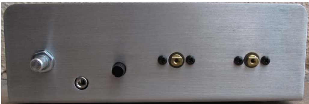
Figure 61. Mount C3 C5 to front panel. Keep screws loose!
