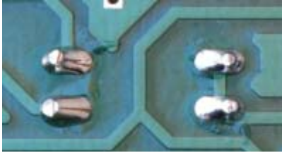
Figure 15. View of trimmed leads after soldering
