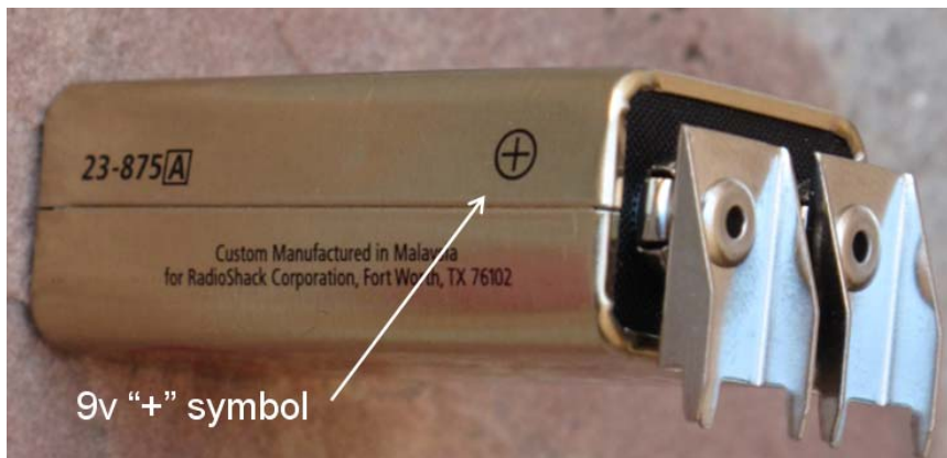
Figure 7. Find the 9v battery “+” symbol as shown above
