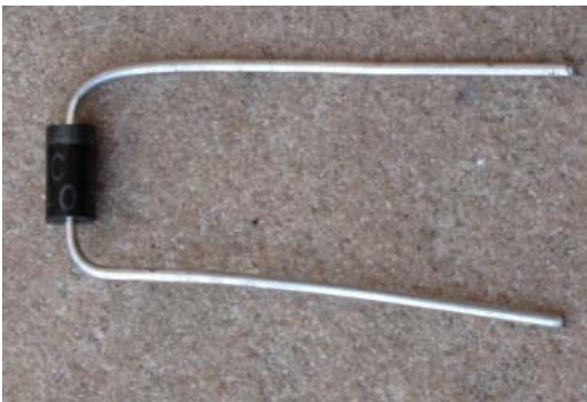
Figure 11. Bend the leads on two of the 1N4004 diodes as shown
