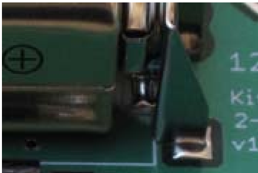
Figure 9. Make sure the battery clip is installed flush to the top of the PC board.
